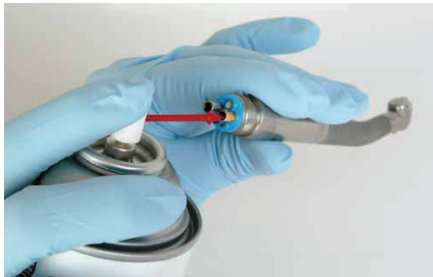
Figure 15. Proper lubrication of handpiece
