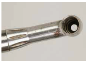
Figure 9. Corrosive effects of sterilization
